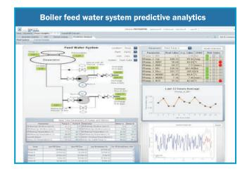
For example, this view provides drill down into one of the systems with visibility into the system parameters for the selected system, in this case - the feed water system.
