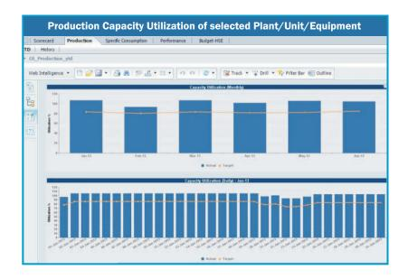
Drill down views provide visibility into multiple aspects of the OEE dashboard. For example, this view shows Performance/capacity utilization with drill down to the plant level and unit level for capacity utilization with a provision to select plant month-wise performance and analyze plant utilization for specific periods.
