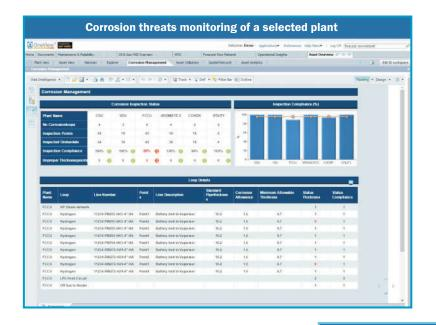
For example, Rolta OneView™ provides visibility into inspection status of corrosion loops in a plant, unit wise, and also provides alerts in case of not meeting the MAT (Minimum allowable thickness) for different equipment, with drill down provisions.
