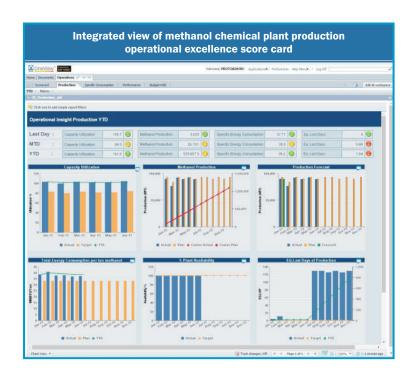
Rolta OneView™ provides an integrated and enterprise level view of chemical production. For example, this view shows methanol chemical plant production that includes key metrics like capacity utilization, production, specific energy consumption, with further drill down, analysis and alarm generation for KPI actual values deviating from plan or budgeted values.
